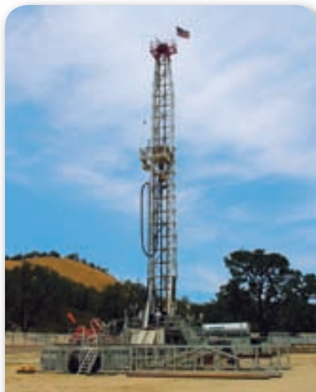
■ Figure 19.26 This drill platform was used to drill a hole 2.3 km deep in Parkfield, California. Once completed, the hole was rigged with instruments to record data during major and minor tremors. The goal of the project was to better understand how earthquakes work and what triggers them. This information could help scientists predict when earthquakes will occur.
